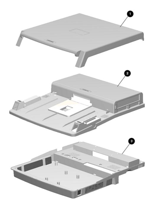
Figure 3-10A. MultiBay-ISA Expansion Base Cover Assemblies
